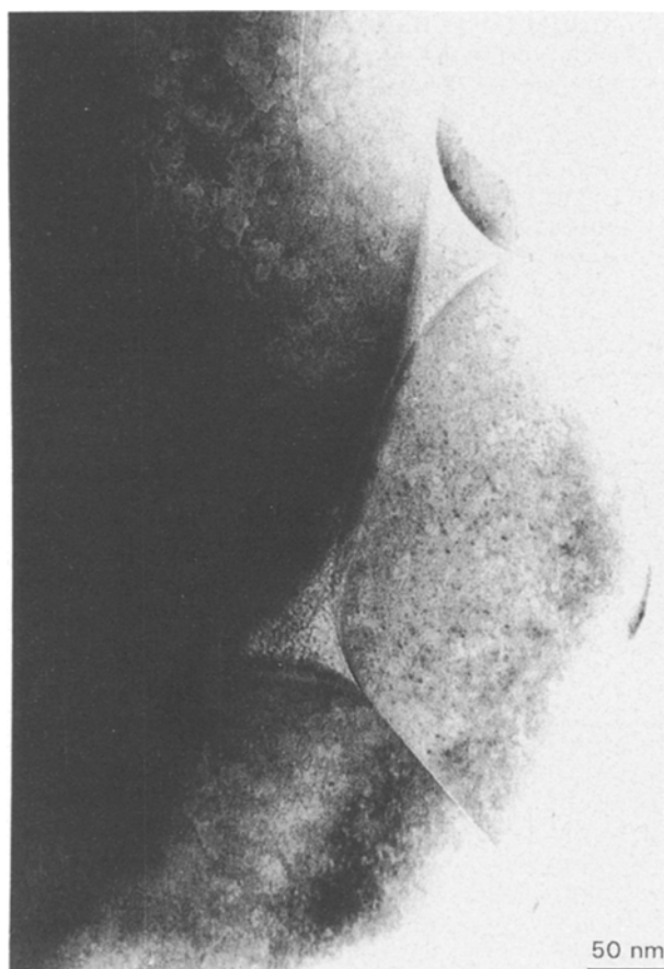
Figure 4 Intergranular phase in a 0.99 SnO 2 -0.01 CuO ceramic sintered in air at 1000 °C for 30 min and quenched at room temperature.
